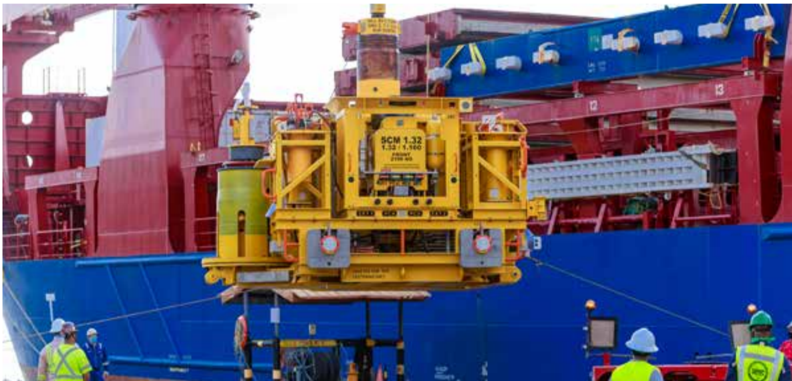
Matapal subsea manifold
